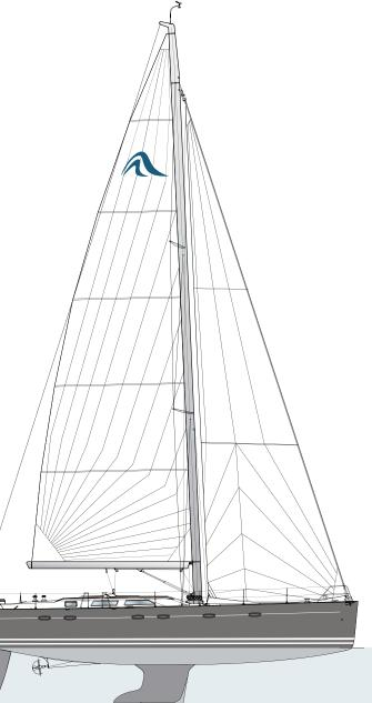
LOA 16.15 m | 53' LWL 14.60 m | 47'9" Hull length 16.15 m | 53' Beam 4.91 m | 16'1" Draft
